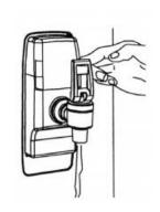
• For filling larger vessels, such as tea or coffee pots, **rotate the lever**180 degrees and pull until it locks into a horizontal position. This allows the vessel to be filled without holding your hand where it may be affected by steam. Boiling water will flow until the lever is returned to its normal vertical position.
